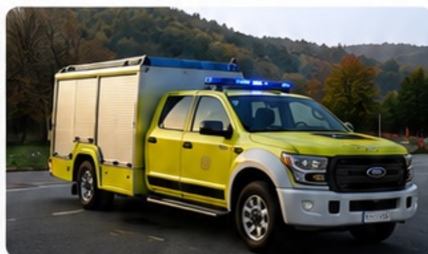
Rapid intervention fire truck equipped with a compressed air foam system
