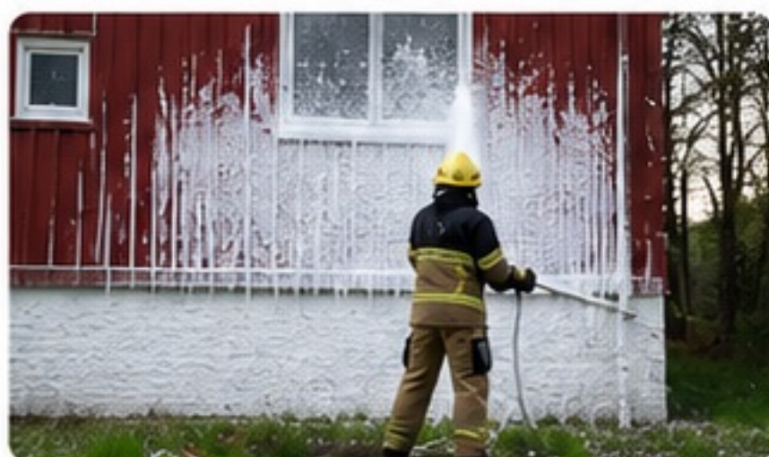
Excellent adhesion performance of compressed air foam
