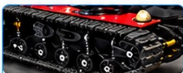
Crawler chassis (6 wheels per side)
